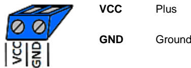
Fig. 2: Power supply connection (blue)
